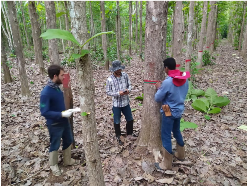
The ONF Brasil team measuring biomass and preparing an annual carbon inventory, following the methodology approved by Verra and recommended by the UNFCCC. Image courtesy of ONF Brazil.
